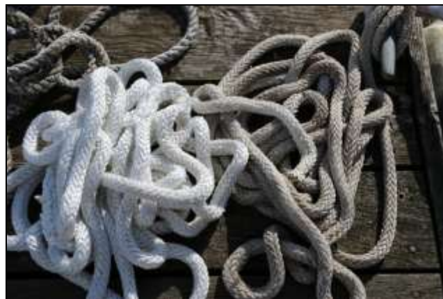
Left: washed dock line. Right: bark dust imbedded dock line.
